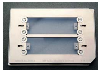
Adapted MALDI plate for cryosections
